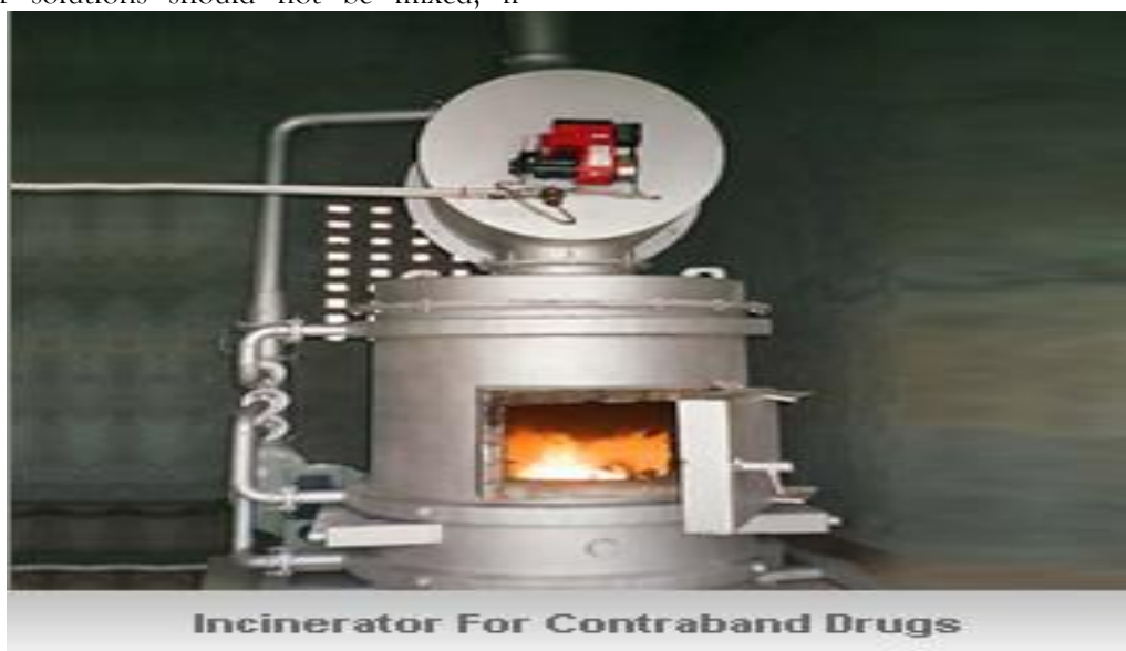
Figure-9 Incinerator for contraband drugs
