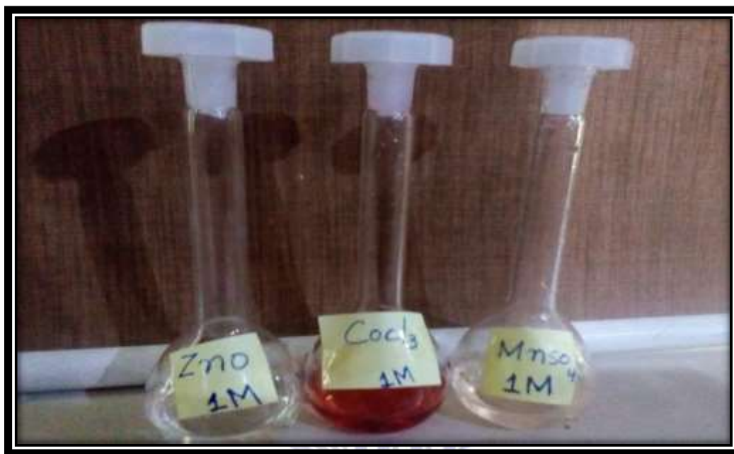
Figure 1.2 Preparation of 1M solutions of ZnO, CoCl 3 and MnSO 4
