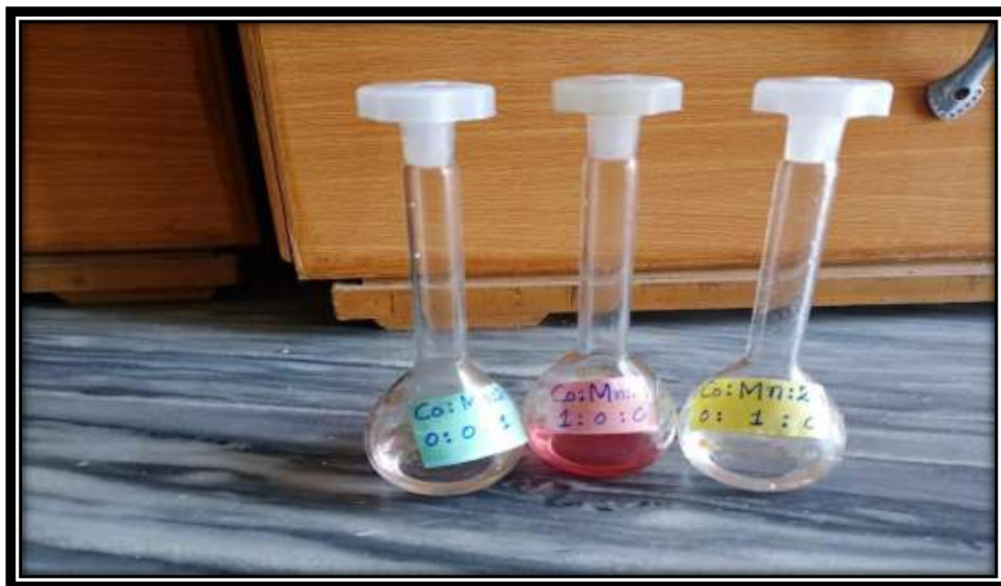
Fig 1.7 Preparation of three reference samples where, Co = Cobalt chloride ( \text{CoCl}_3 ), Mn = Manganese sulphate ( \text{MnSO}_4 ), and Zn = Zinc oxide ( \text{ZnO} )
