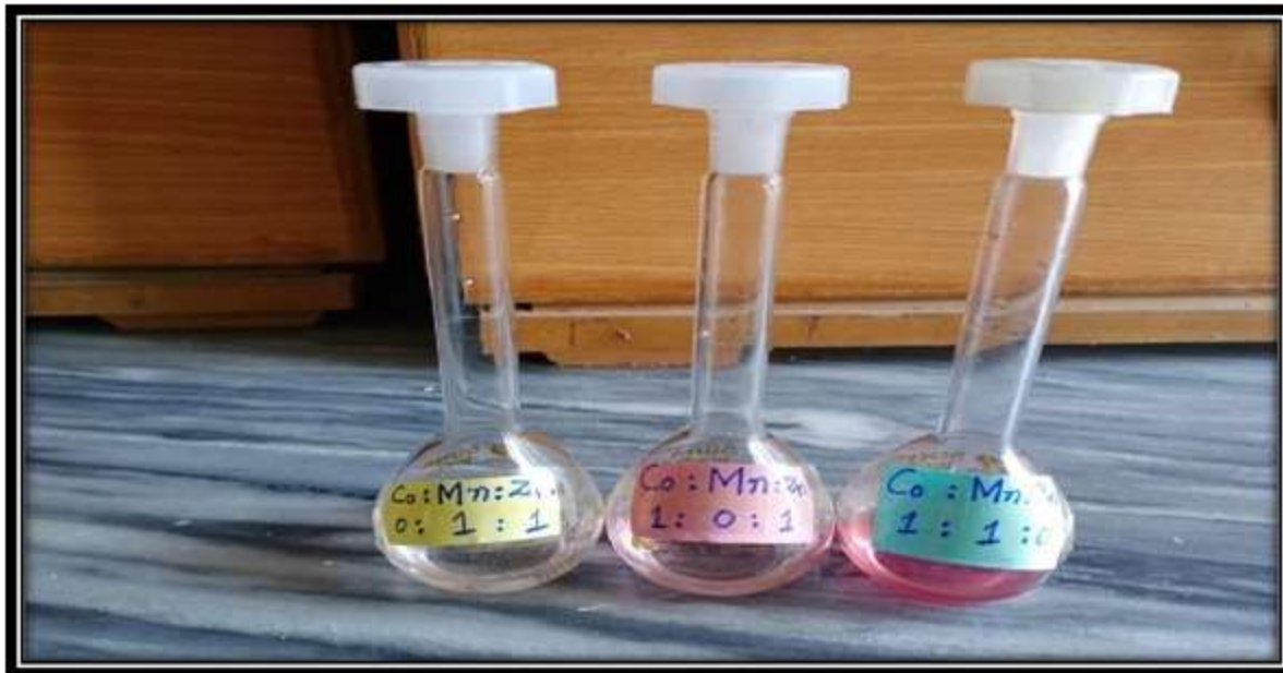
Fig 1.9.Preparation of three test samples where, Co = Cobalt chloride ( \text{CoCl}_3 ), Mn = Manganese sulphate ( \text{MnSO}_4 ), and Zn = Zinc oxide ( \text{ZnO} )
